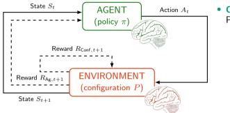
Configurable Markov Decision Process (Conf-MDP) 1 Observe the state  $S_t$ 2 Perform an action  $A_t \sim \pi(\cdot|S_t)$ 3 Transition to the next state  $S_{t+1} \sim P(\cdot|S_t, A_t)$ 4 Agent obtains reward  $R_{t+1,Ag} = r_{Ag}(S_t, A_t, S_{t+1})$ 5 Configurator obtains reward  $R_{t+1,Conf} = r_{Conf}(S_t, A_t, S_{t+1})$
